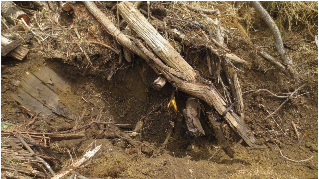
Photograph 2: View of the logs and tree debris observed at TP-2.
