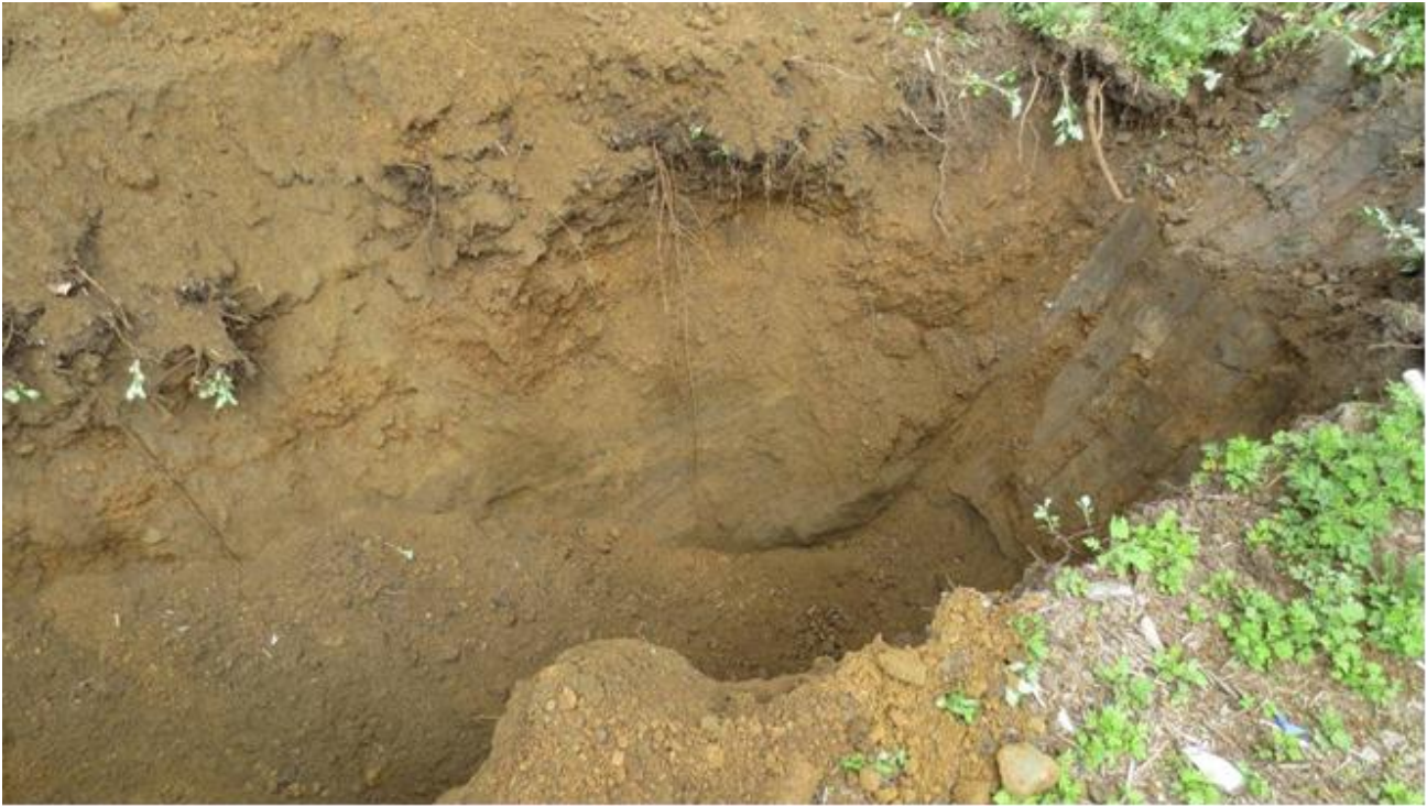
Photograph 5: View of the native sand observed at TP-4.
