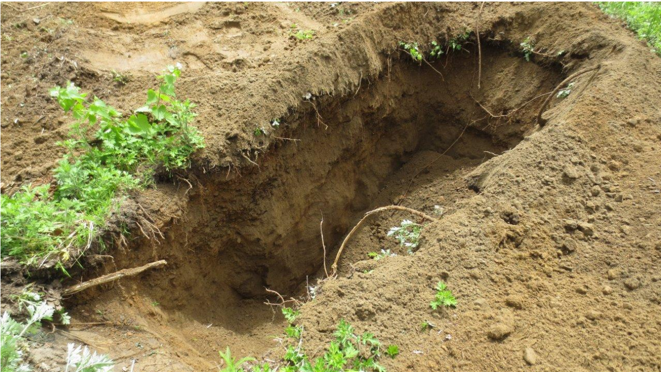
Photograph 6: View of the native sand observed at TP-5
