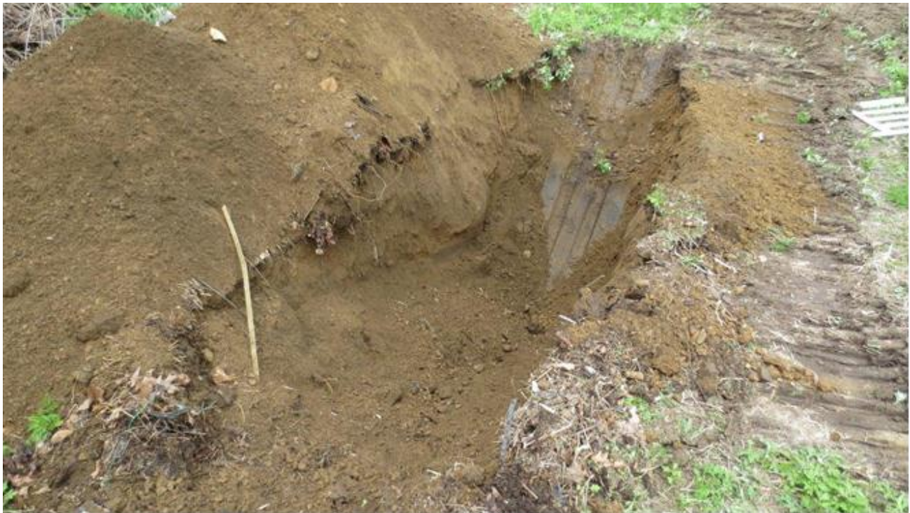
Photograph 7: View of the native sand observed at TP-6.
