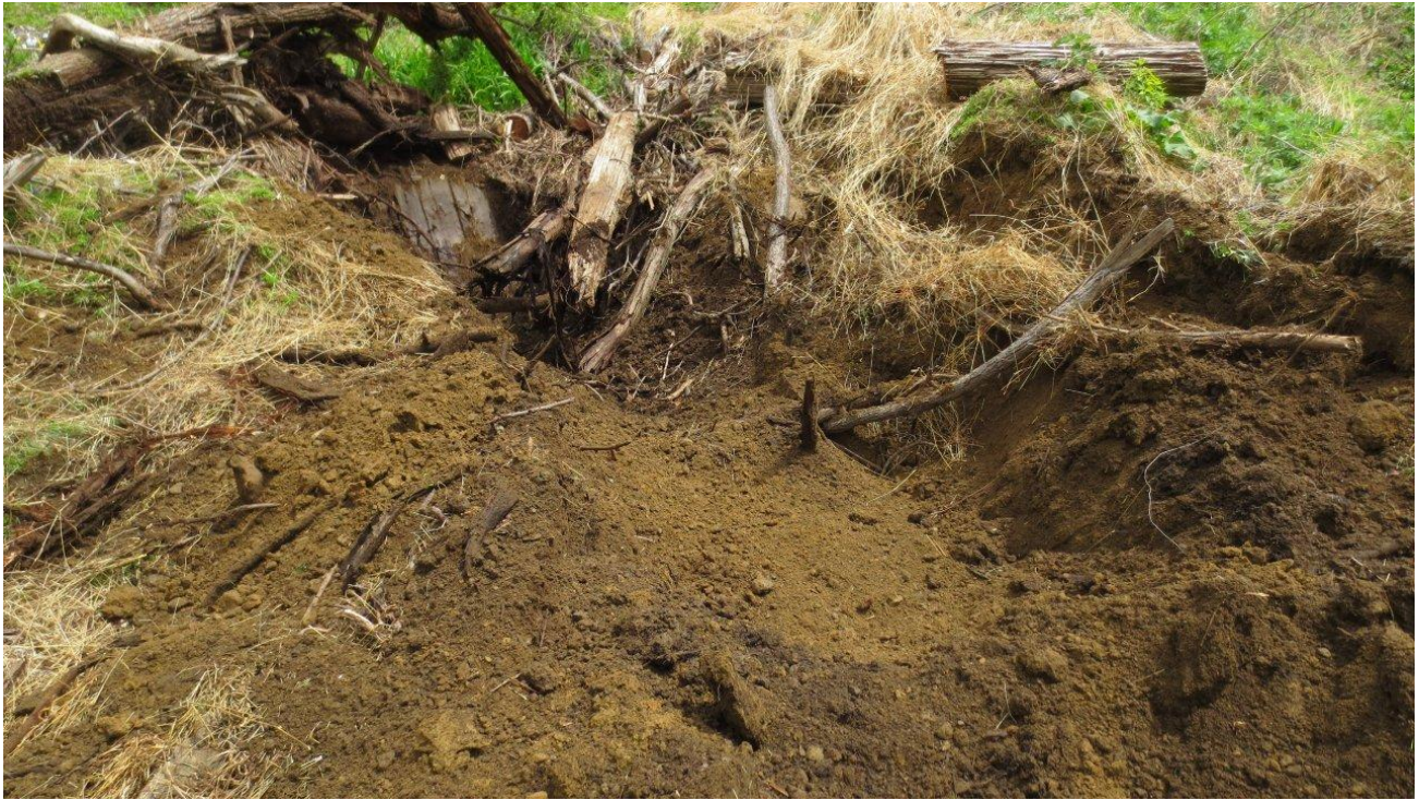
Photograph 3: Additional view of the tree debris observed at TP-2.
