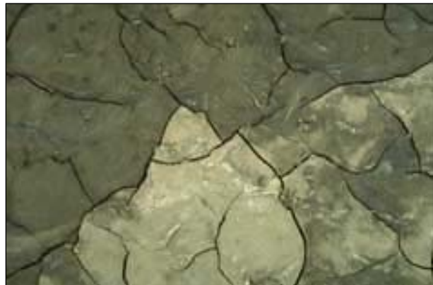
Figure 5. 15 Shows typical compacted soils that nearly reach the bulk density of concrete (Schueler et al 2000)
