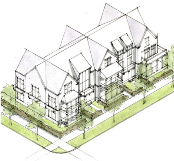
Contemporary touches in openings and façade composition can help to distinguish one multi-family address from another.
