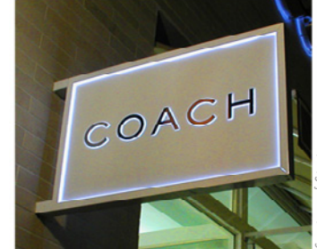
Edge and halo illuminated projecting blade sign
