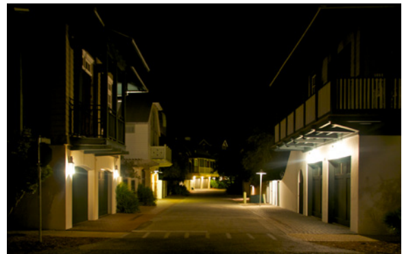
Architectural lighting outside the Resort Core should minimize light spill onto neighboring buildings, trees, or other features.
