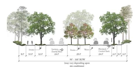
AASHTO design criteria for thirty (30) mph roadways and, where possible, have been situated along similar alignments of the existing roadways. The new roadway designs will potentially require bridge improvements and/or replacements in two locations (Kiamesha Creek intersections with Thompsonville Road and Chalet Road) to accommodate for utility infrastructure upgrades and widened roadway cross-sections.
