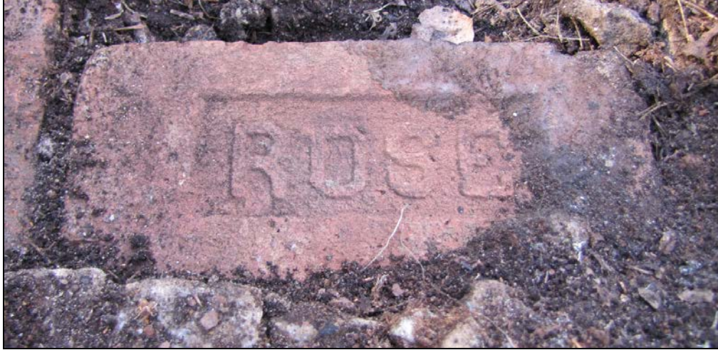
Photo 35: Closeup of frog panel showing "ROSE" from the Roseton brickworks on the Hudson River.
